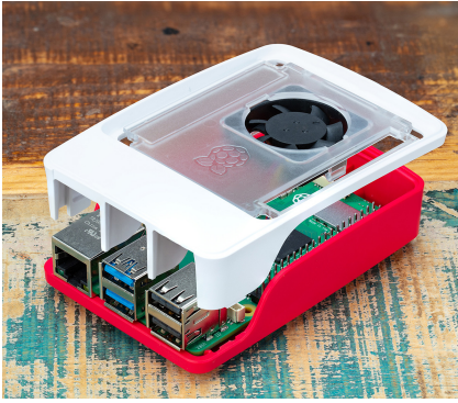
Figure 2-7 Attaching the fan assembly and frame
