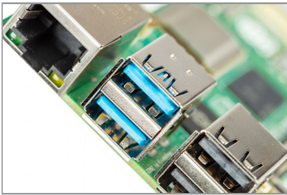
Figure 1-7 Raspberry Pi's USB ports
