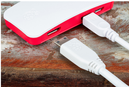
Figure 2-15 Connecting the HDMI cable to a Raspberry Pi Zero
