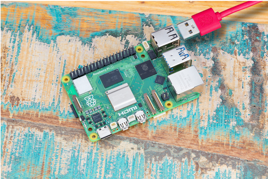
Figure 2-14 Plugging a USB cable into a Raspberry Pi 5
