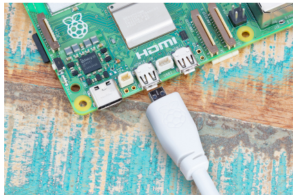
Figure 2-16 Connecting the HDMI cable to a Raspberry Pi 5
