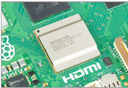
Figure 1-2 Raspberry Pi's system-on-chip (SoC)
