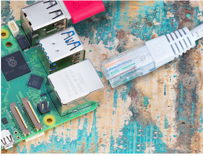
Figure 2-17 Connecting Raspberry Pi 5 to Ethernet
