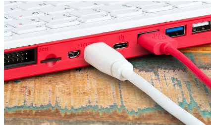
Figure 2-22 Connecting the HDMI cable to a Raspberry Pi 400
