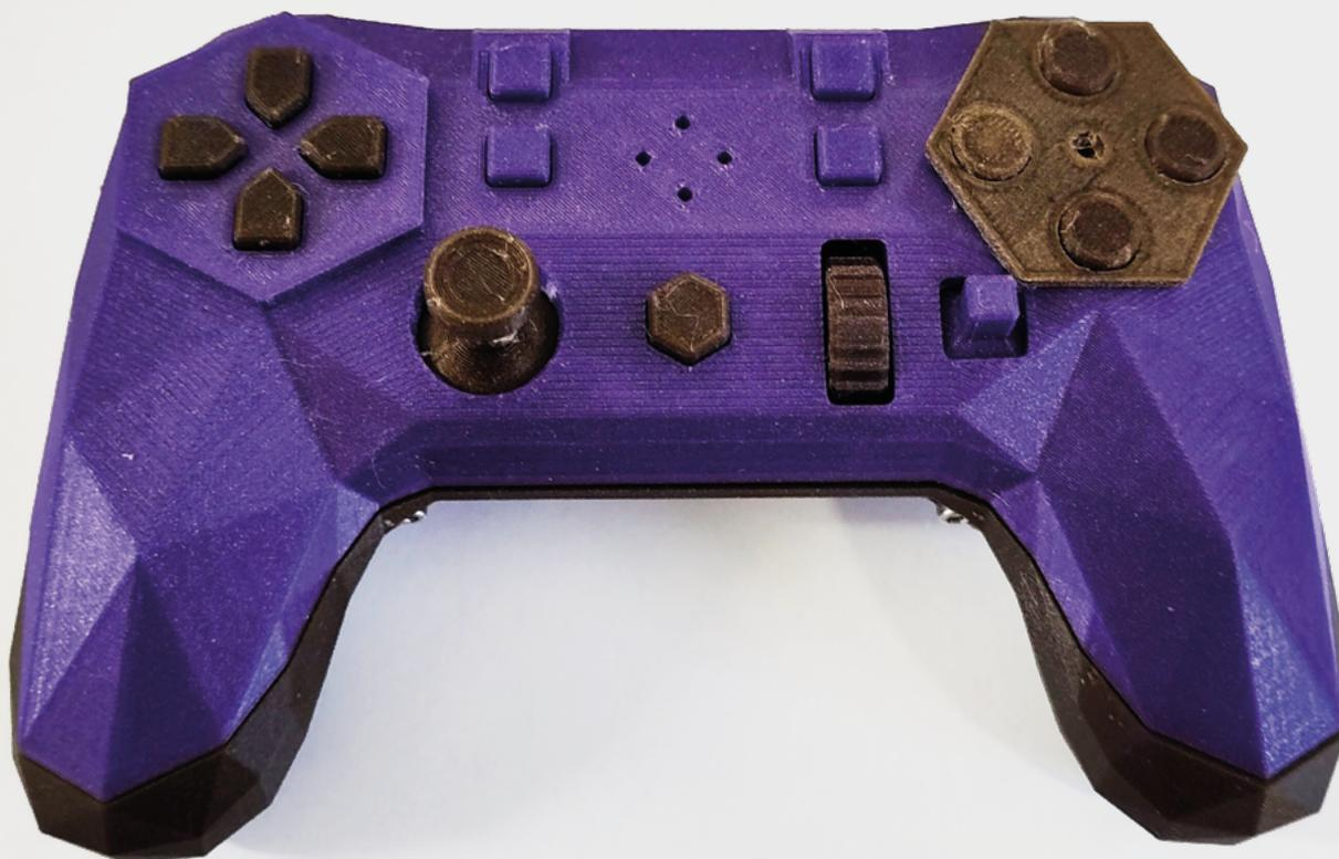
parts together. It took some shaving, sanding, and a bit of lubricant to get everything moving nicely. The problem's made worse by the fact that some of the switches that move the 3D-printed parts have very little push-back, so unless everything is moving freely, the buttons will stick. If you're thinking of building one, we'd recommend printing out a few of the parts (perhaps the bottom section and the trigger buttons), and see how the tolerances work on your printer.
