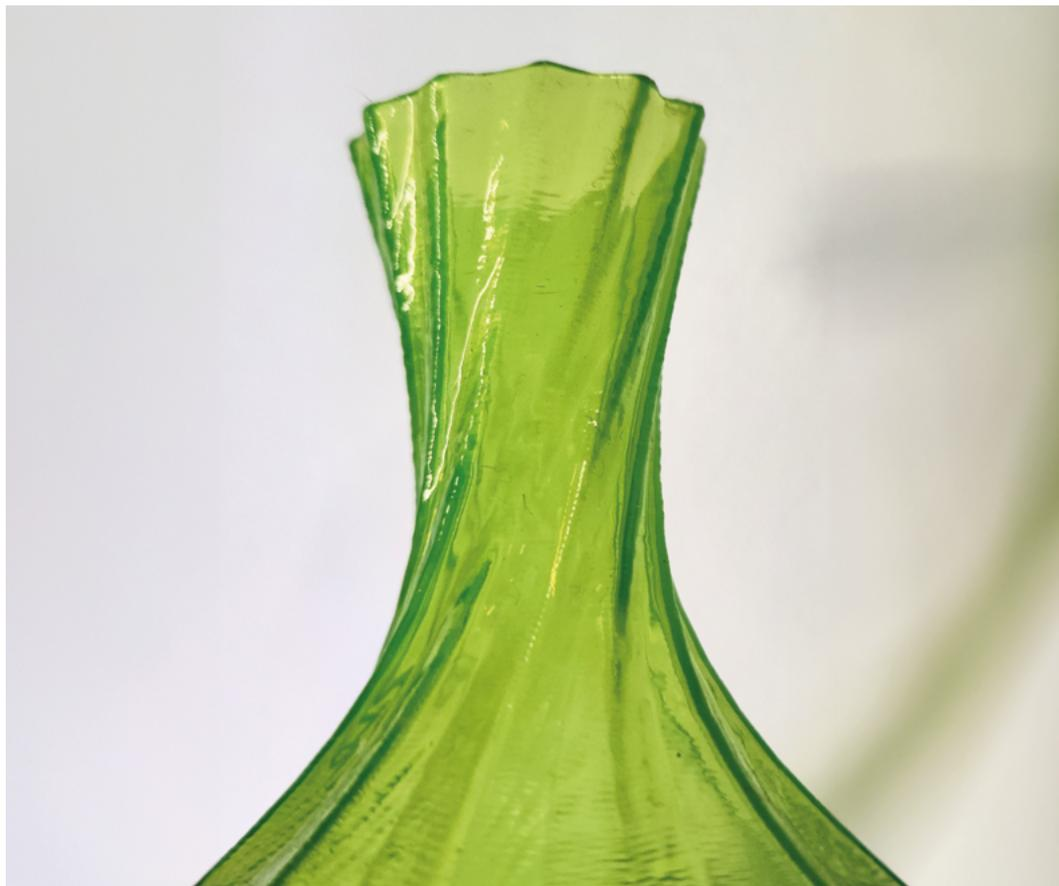
**Left** ♦ We heavily smoothed this one and the layers are only just visible. However, it has distorted the vase slightly. Corners are more rounded and finer detail is lost
