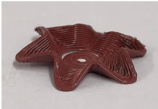
**Figure 1** ♦ This spacer doesn't have layers in the traditional sense – the print head moves round while going up and down
