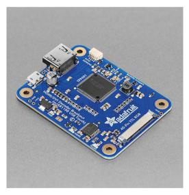
he TFP401 HDMI/DVI Decoder is a small board that serves a useful purpose. Now you can easily add a 40-pin TTL/TTF display, via HDMI/DVI video, to a Raspberry Pi project. What makes this board a little more unusual, other than its diminutive size, is the addition of an AR1100 USB resistive touchscreen driver. You can power the board over USB and send the signal out to a small 40-pin TFT display.
