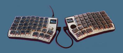
Each keycap has a tiny OLED, so can easily be relabelled if needed
