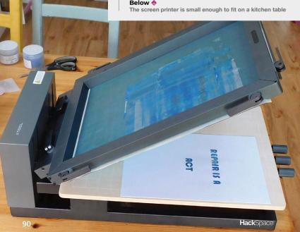
Screen printing has been around for a long time. The basic idea is that you have a fine mesh of fabric. You cover most of this mesh with some sort of impermeable barrier, but the bit where you want ink (or paint) to get through, you leave uncovered. You then hold this screen against the thing you want to print onto and squeegee the ink (or paint) through it. If all goes well, you should have a perfect replica of your design on the surface below.
