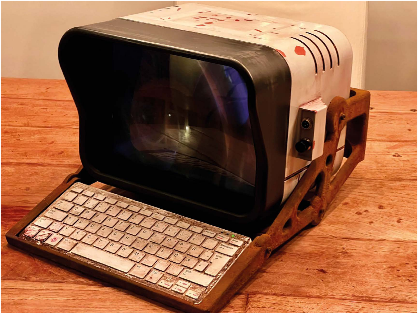
Left ♦ The case was printed in two halves to fit on Rick's 3D printer, then glued together using epoxy.
