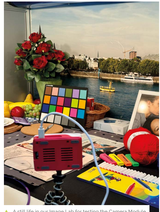
▲ A still life in our Image Lab for testing the Camera Module
