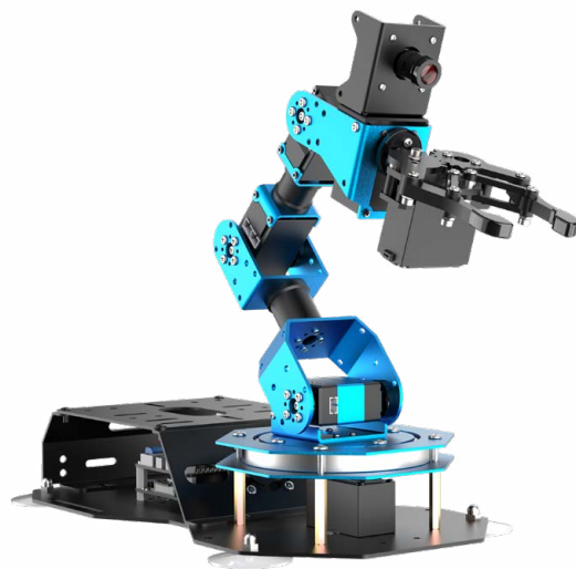
▲ Block-stacking makes use of computer vision and image recognition via Raspberry Pi
