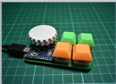
HotKeys v2 ♦ Rotary encoders are often included in mechanical keyboards, for the scrolling of pages etc. This one is in a programmable macro keypad
