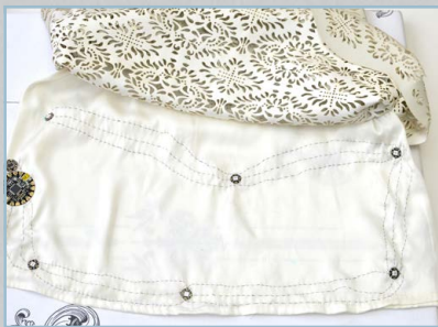
Sparkle Skirt ♦ Conductive thread is great for connecting components in wearable projects such as this light-up sparkle skirt controlled by an Adafruit FLORA microcontroller
