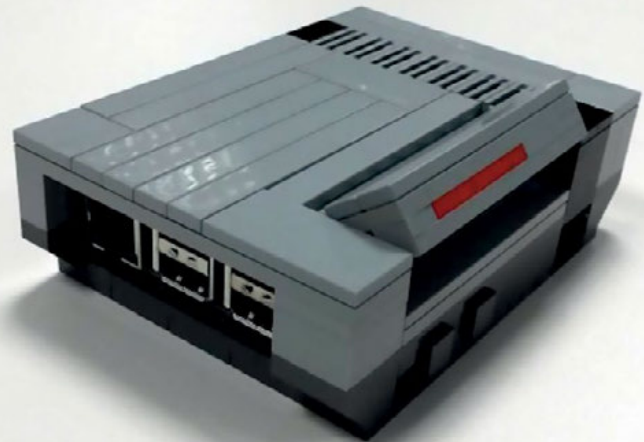
Putting the parts together results in this Raspberry Pi case. It looks like a classic NES console, but with access to the Raspberry Pi ports. The lid (used for cartridges in the original NES) provides access to the GPIO pins
