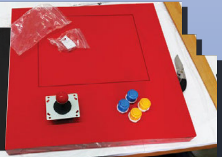
A square in the table is cut to contain the 17-inch display. The wood is then prised out to reveal the structural filling inside
