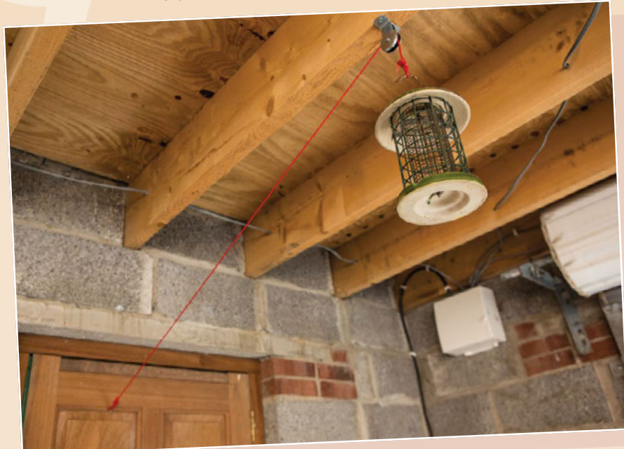
Left The door is connected to a weight via a pulley system. When the actuator moves back, the door automatically swings open
