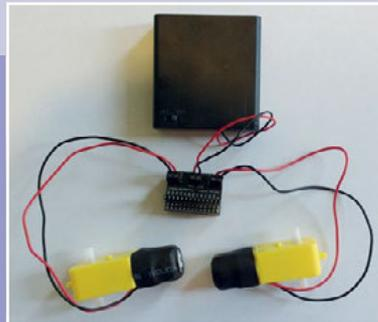
If your left and right are mixed up you can swap wires on the motor control unit or change GPIO values in the **robot** variable:
