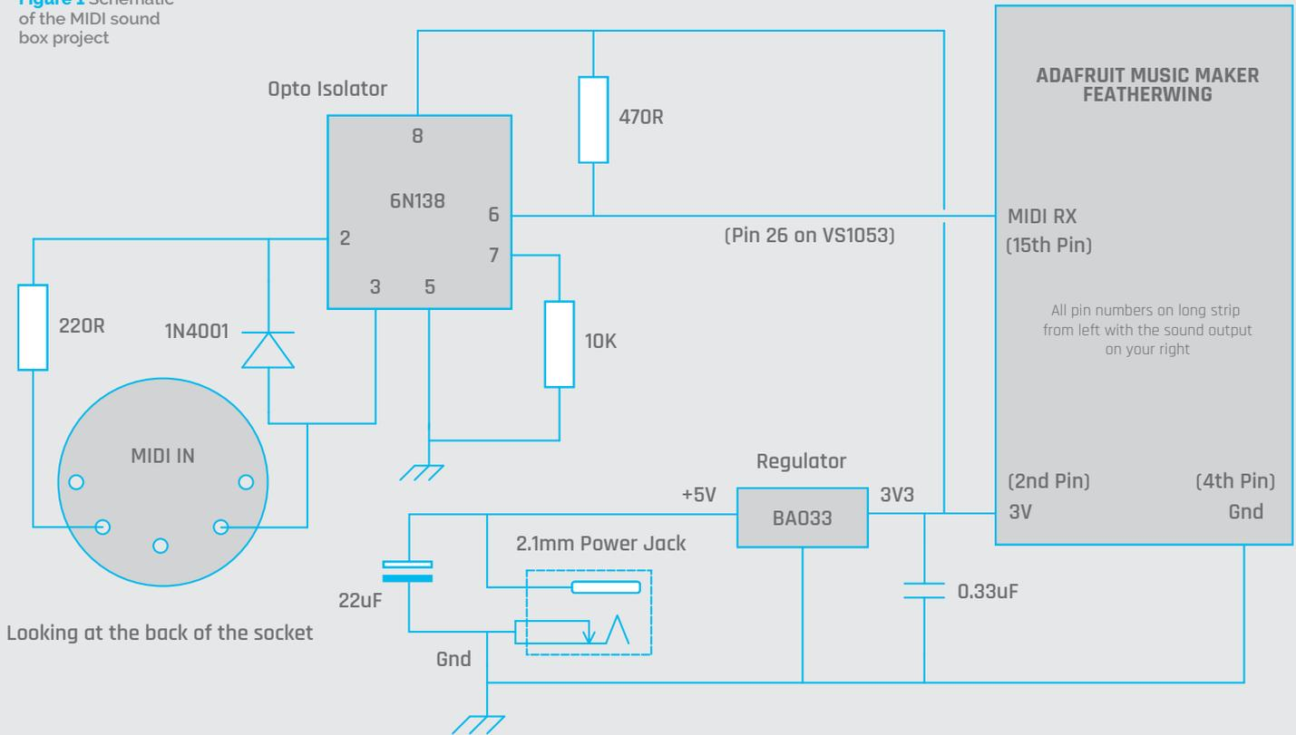
round), and also a current-limiting resistor for the LED inside the optical isolator. On the output side, a Darlington transistor pair picks up the infrared light from the LED and amplifies it. This signal can then be sent to the MIDI input of the VS1053. We need to feed the board with 3V3, so we have included a voltage regulator to do this.
