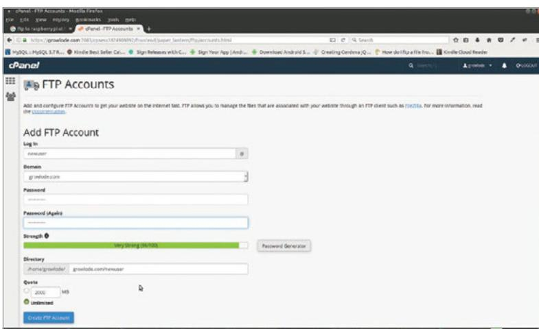
the same remote server, that takes more work. To do that, we can create FTP accounts for each Raspberry Pi monitoring a remote garden. Then, each Pi will authenticate and upload the file to its own account.
