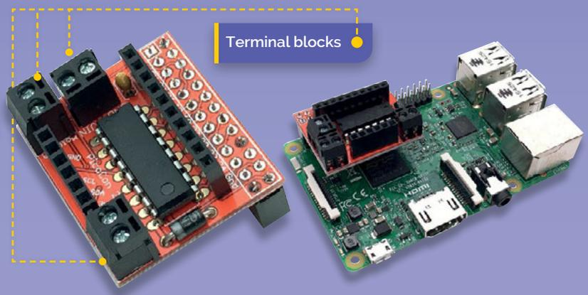
pack must be connected so that the red wire goes into port labelled VIN. The black wire goes into the port labelled GND. Make sure the battery pack is turned off when you do this. The motors can be connected to their terminal blocks any way around. Then tighten the screws again.
