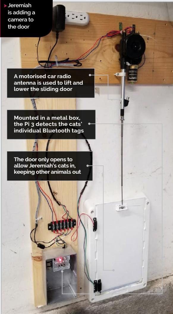
A motorised car radio antenna is used to lift and lower the sliding door
