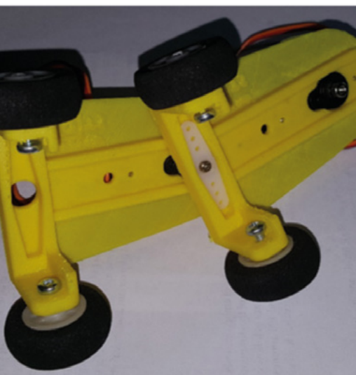
Above ♦ One segment assembled and ready to be inserted into the worm
