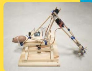
Once again, this is all powered by Arduino, but controlling motors and servos with Raspberry Pi is incredibly easy using various motor or robotic HATs. Pairing a game controller will be a bit easier as well. The potato counterweight is universal, though.
