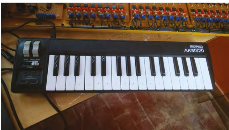
▲ A MIDI keyboard is connected to the setup, enabling a user to play live and record songs
