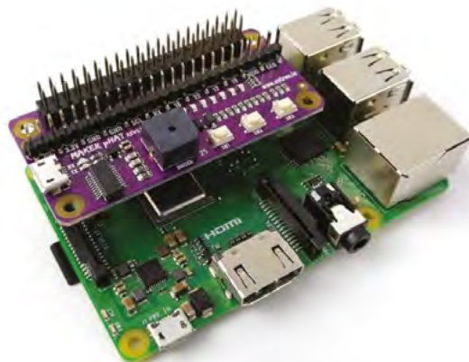
▲ The supplied stacking header provides full GPIO breakout and can be used to elevate the board on a full-size Raspberry Pi
