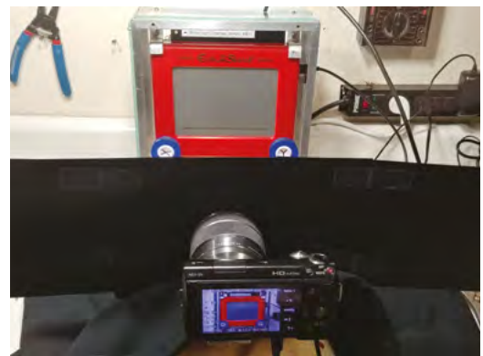
▲ For the creation of stop-motion videos, the camera sits behind black fabric to prevent reflections, and each image is drawn 1 to 2mm apart for smooth footage
