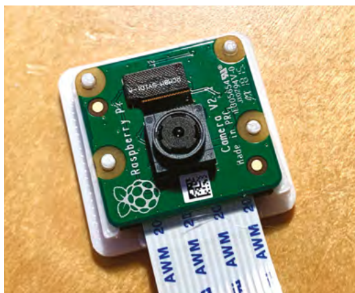
▲ The official Raspberry Pi Camera Module is a perfect choice for this project
