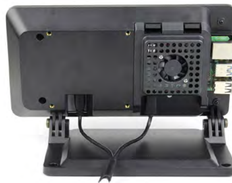
▲ The additional case fan and vents can be handy for intensive loads
