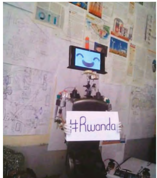
▶ Joseph's first ever robot, TIM, made from a TV antenna, with facial expressions by Google Assistant on an old mobile phone
