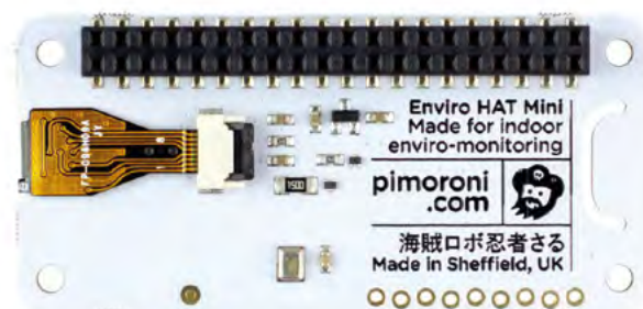
▲ The rear of the board, showing the pre-soldered female GPIO header
