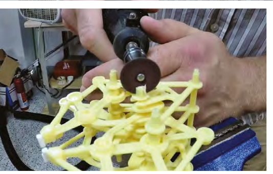
Above ♦ A rotary tool is great for making little modifications to plastic kits
