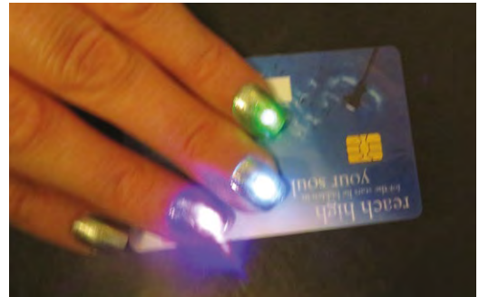
Above ♦ NFC nails lighting up when a contactless bank card is being read
