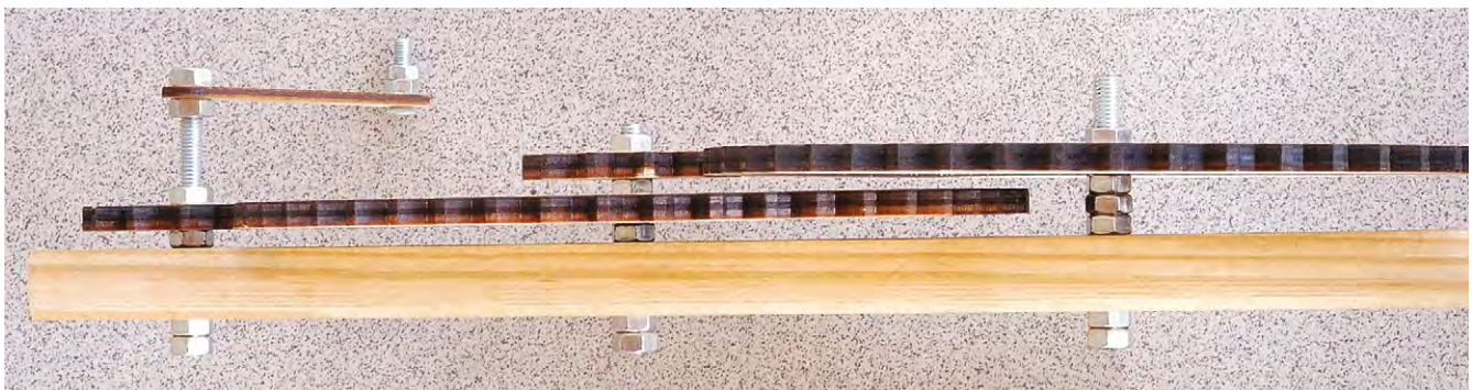
Below Side view showing vertical orientation of the gears. The large gear on axle 3 rests on three M6 nuts
