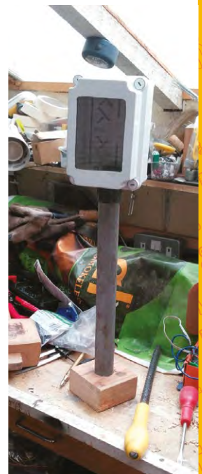
Below ♦ An IP67-rated box should keep water out
