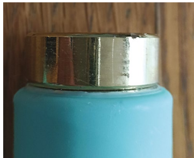
Above ♦ The head of this hammer is made from brass which absorbs some of the shock and also helps prevent damage to stamps
