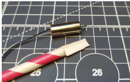
Figure 4 ♦ The start point of a power pod is to cut a section in the straw to mount the motor in
