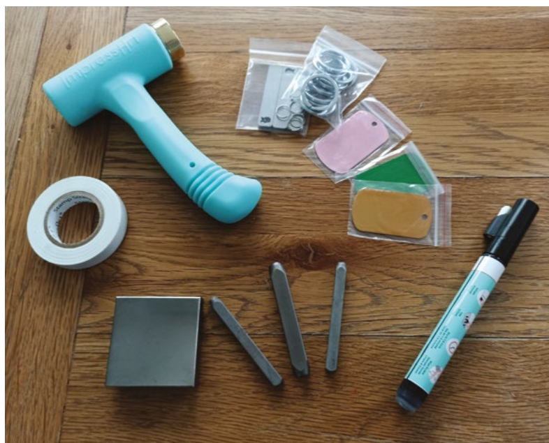
Above ♦ A selection of the tools and consumables required for metal stamping. Some kind of sticky tape, or washi tape, is extremely useful in order to hold the blank in place on the block while you stamp
