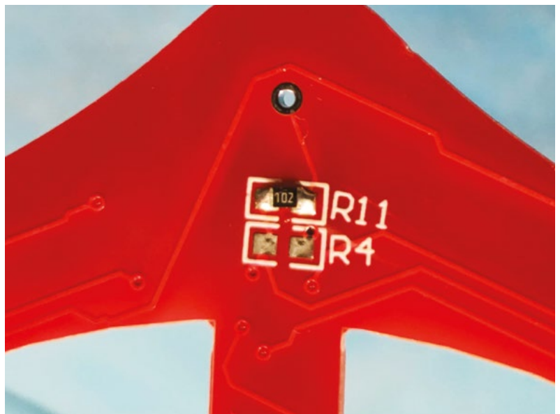
Left ♦ Make sure you're happy with the placement before soldering the second joint
