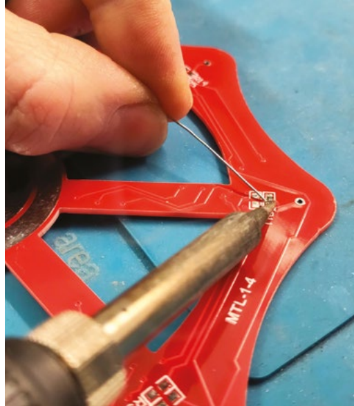
Above ♦ You only need the slightest bit of solder on the pad – it's not there to fill a gap, just make an electrical connection with the resistor
