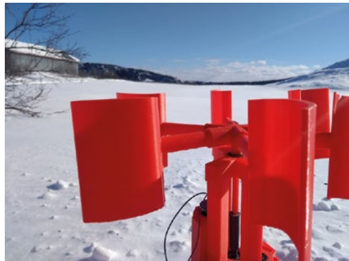
Left ↙ The single-stage setup can produce up to 100 watts of power
