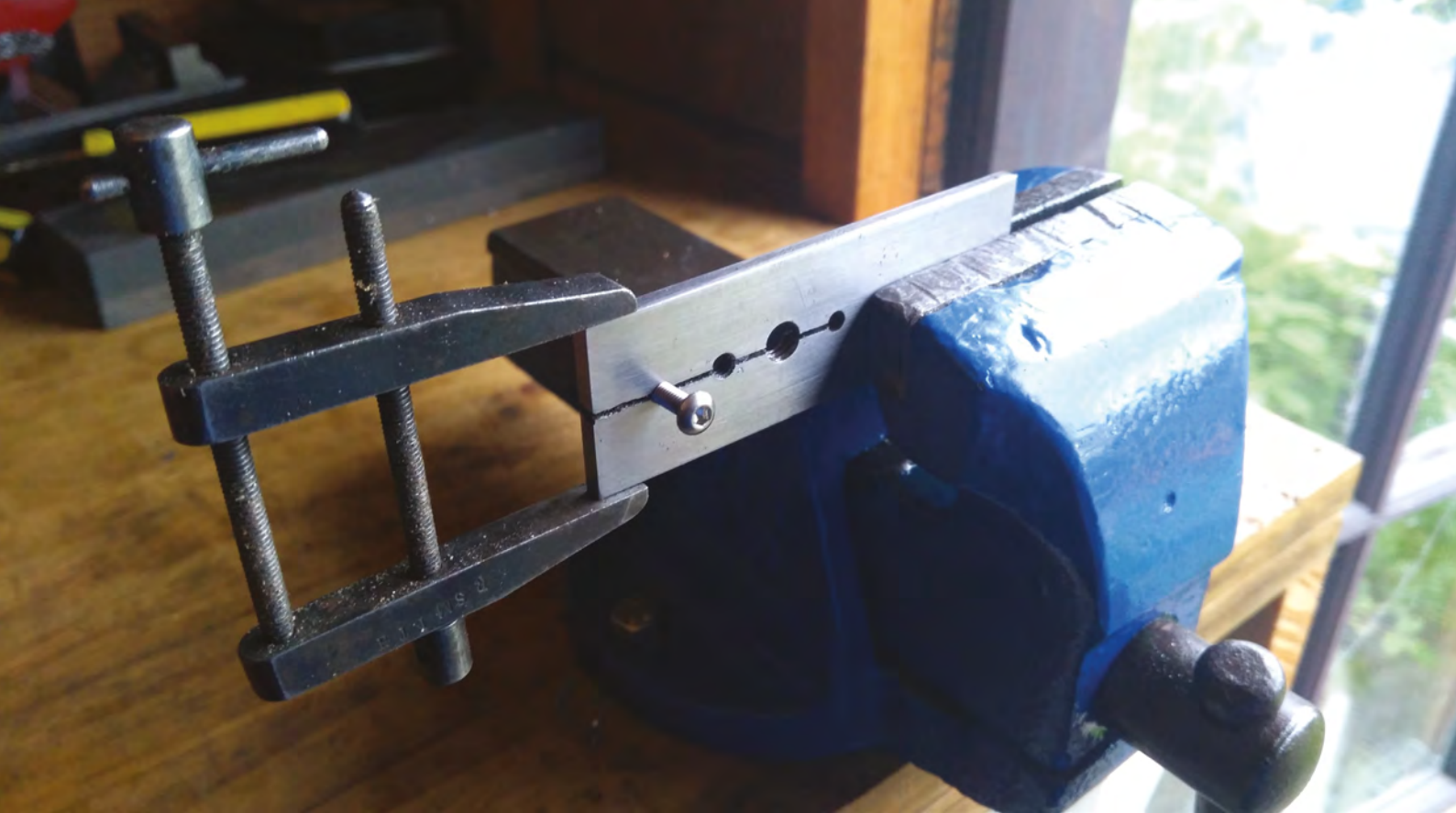
Figure 6 ♦ Using a vice and additional clamp to change the orientation of the workpiece held in the stud clamp
