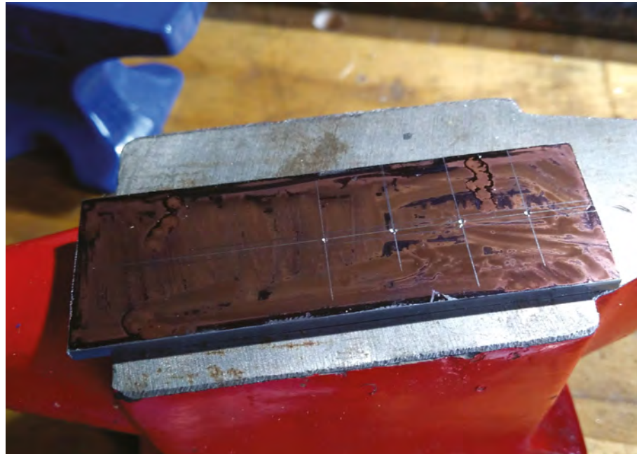
Figure 2 ♦ The workpiece, marked and punched ready for drilling
