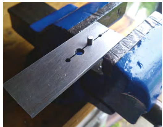
Figure 5 ♦ Using the stud clamp in a vice to hold a small threaded bar securely, allowing the end of it to be filed square
